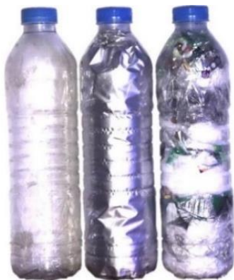
Figure 3: Empty PET bottle (left), bottle filled with LAFs (middle), and bottle filled with assorted plastic bags (right).
