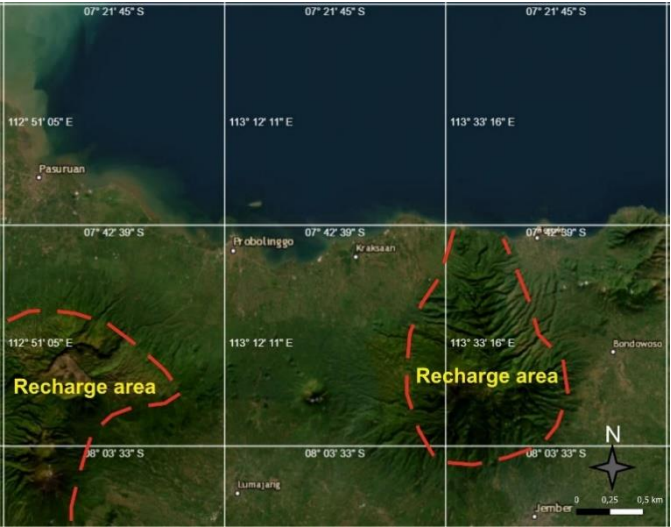
Figure 5: It can be estimated that the natural recharge processes are derived from the northeast slope of the Bromo-Tengger volcano and the northwest slope of the Iyang-Argopuro volcano, which consist mainly of lava flow complexes with middle-high permeability (modified from (Hendrayana et al., 2024)).
