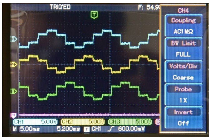
c) Oscillogram of the output voltage of the experimental 6 kW inverter during testing
