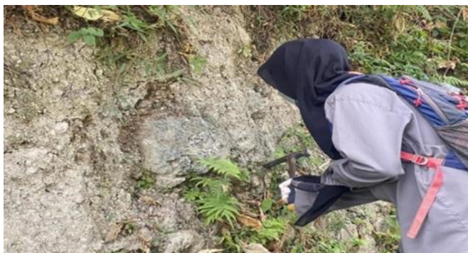
Figure 4: Overburden rock sampling at Kandi area
