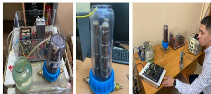
Figure 4: Laboratory Model of a High-Voltage Electric Discharge System for Water Treatment in the Kapshagay Reservoir
