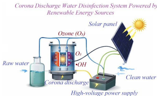
Figure 3 : Structural diagram of a corona discharge water disinfection system powered by renewable energy sources
