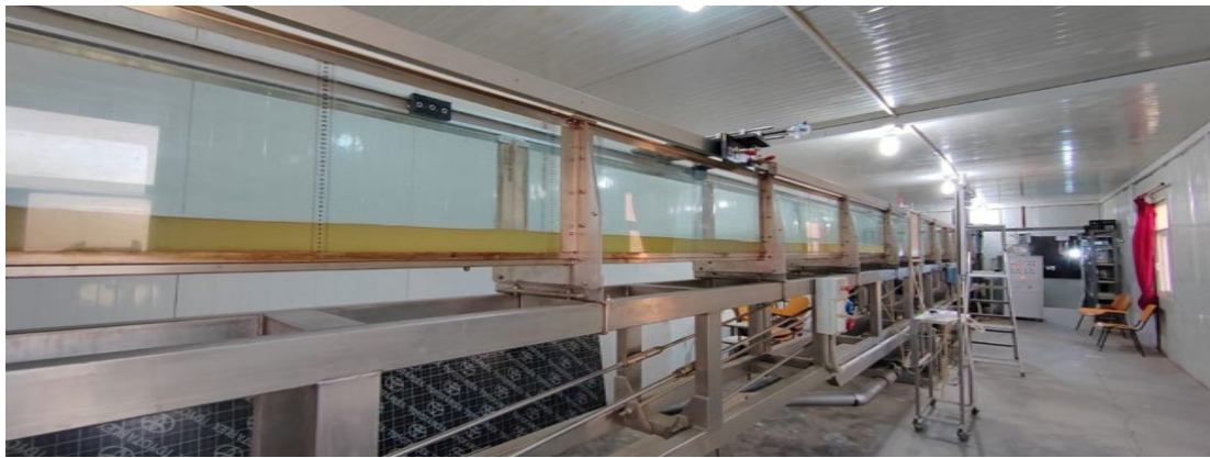
Figure 3: The laboratory flume
