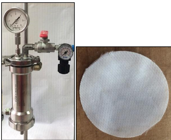
Figure 1: Laboratory scale Nutsche filter (left) and filter medium (right)
