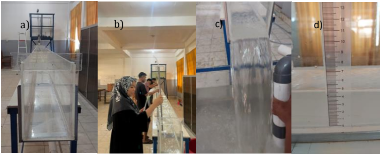
Figure 2: (a) open channel, (b) velocity height measurement, (c) discharge, (d) water level
