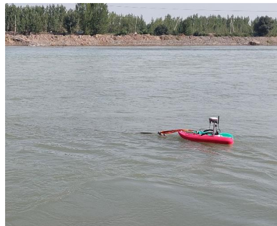
Figure 1: Measurement of hydraulic parameters of river flow using the SonTek RS5 Doppler device (based on fieldwork conducted between May and August 2024)
