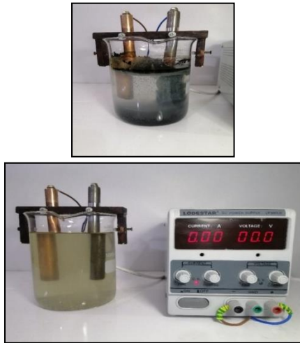
Figure 3: Wastewater samples using electrodes (Cu-, Fe+) and voltage 30.
