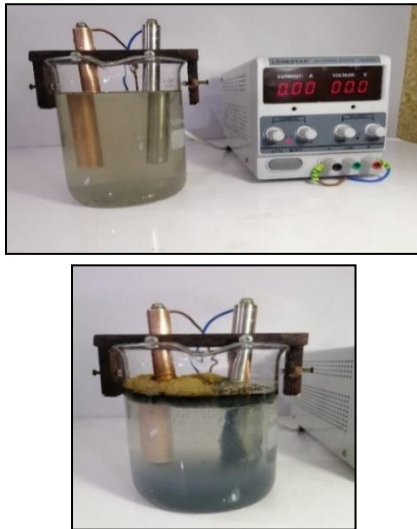
Figure 4: Wastewater samples using electrodes (Cu-, St. St+) and voltage 30.
