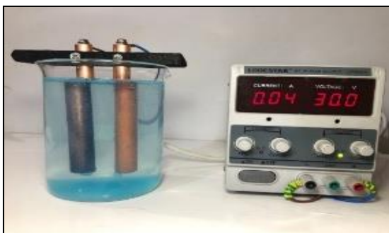
Figure 6: Determine the optimum pH at concentration=10 ppm, d=2cm, voltage 25.
