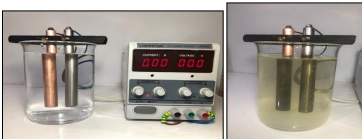
Figure 8: Determine the optimum distance between electrodes at PH =9 at concentration =10 ppm, voltage 30.
