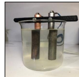
Figure 7: Determine the optimum voltage at pH =9 at concentration =10 ppm, d=2cm
