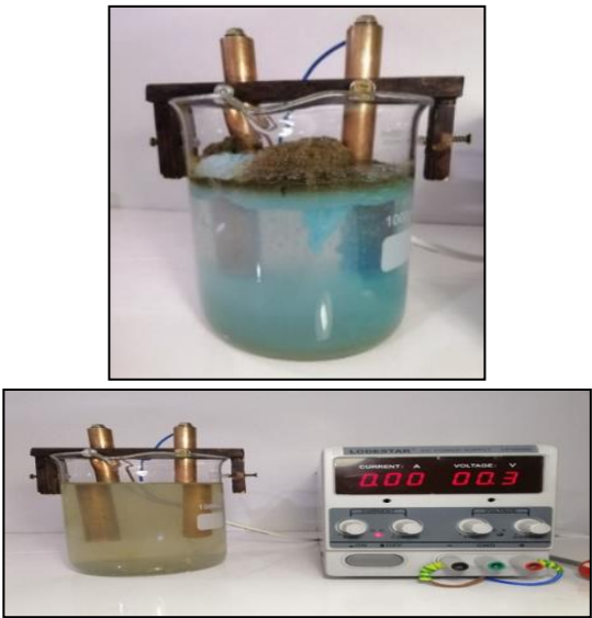
Figure 2: Wastewater samples using electrodes (Cu-, Cu+) and voltage 30.
