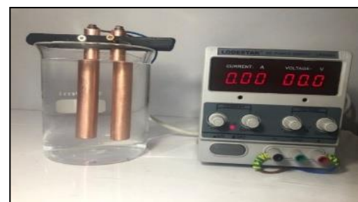
Figure 7: Determine the optimum voltage at pH =9 at concentration =10 ppm, d=2cm
